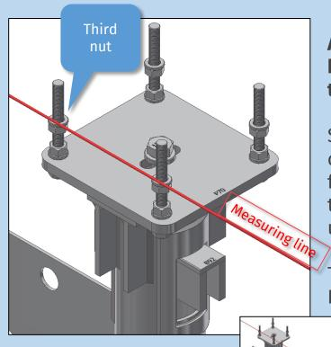
Adjustment of the correct height before mounting the post.
