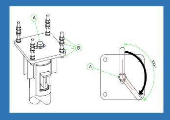
Angle routing can be done by hand or machine, the main thing is that the correct angle is achived::
